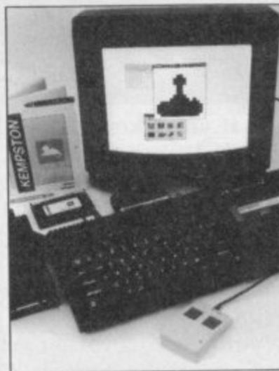
The KEMPSTON MOUSE consists of: High resolution 2 button mouse, mouse interface, Toolkit software and manual.
